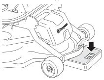
3 Adjust the cutting unit's ground pressure by screwing the adjuster screws, which are located behind the front wheels on both sides, in or out. The ground pressure should be between 12 and 15 kg and the springs evenly tensioned.
